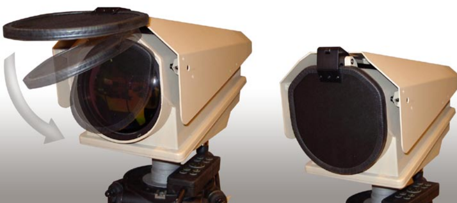
The protective lens cap of the HRC can remotely be positioned before the lens to protect it.
